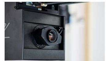
Camera system with a CMOS-based line sensor.
